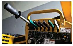
ROTATING OPERATOR'S STATION. Along with the attachment controls, the operator's station can manually rotate 90 degrees.
