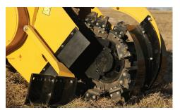
TRENCHER ATTACHMENT. The trencher attachment in this RTX750 SOC can cut a 60.9-cm (24-in) wide by 91.4-cm (36-in) deep trench. The sliding trencher moves from the center to 40.6-cm (16-in) to the left and the height can be adjusted for convenient transport.
