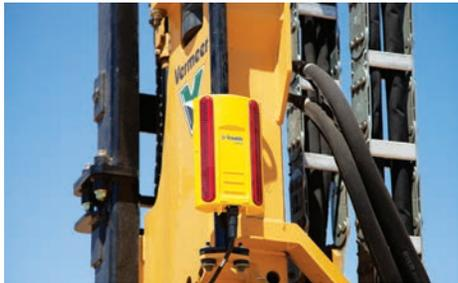
**IMPROVE YOUR ACCURACY.** An optional laser receiver integrated into the control system and a GPS-compatible design (capable of accepting compatible third party systems) can help improve productivity.
