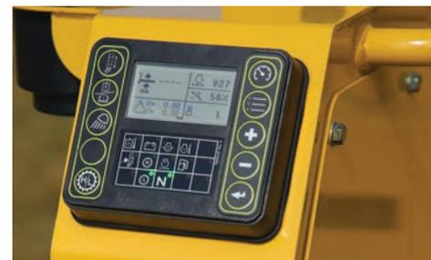
**AT YOUR FINGERTIPS.** An industry-unique on-machine control system offers the operator a variety of machine information, including pile angle and height. Display also shows machine maintenance reminders to help maintain service schedules.
