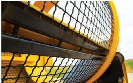
**PRODUCT VARIETY.** Change product size efficiently with the quick-change screen design. Five large bolts adjust a tensioning hook to allow operators to quickly change screen sizes.
