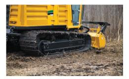
**TRACK OPTIONS.** With the option of either steel or low ground pressure (LGP) tracks, operators can choose which style fits their jobsite needs. With the weight of the mulcher head calculated in, the total machine weight is centered on the tracks resulting in even weight distribution and lower ground pressure.
