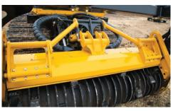
**SELF-POSITIONING DEFLECTOR.** The patentpending self-positioning thrown object deflector helps direct thrown material at a consistent discharge angle, regardless of head position.
