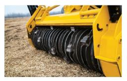
**ROTOR PERFORMANCE.** The externally balanced, ringed rotor helps guide material to the cutting tips for a more clean cutting path while also controlling the depth of cut. Interchangeable tip options allow operators to customize cutting performance to meet their jobsite needs.
