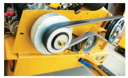
THE CENTRIFUGAL CLUTCH engagement prevents belt slip when engaging the clutch which means fewer maintenance costs.
