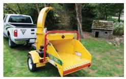
THE LARGE INFEED OPENING 6 in x 8 in (15.2 cm x 20.3 cm) makes feeding irregular material easier and decreases the amount of saw cuts needed prior to feeding the chipper.
