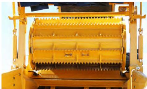
**ENHANCED INFEED.** The feedroller planetary is fully enclosed for protection from debris and offers a tighter clearance between the feedroller and mill housing, helping reduce material blockage and drag on the feedroller circuit.
