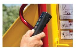
**OPERATOR CONTROL.** The Tree Commander<sup>™</sup> remote control comes standard with the AX19, and an optional full-function remote is available. The operator is able to control the functions of the brush chipper remotely to improve jobsite productivity.
