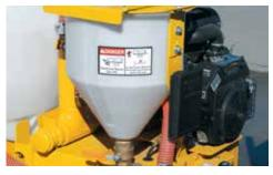
**KEEP IT MIXED.** A hopper with a round design and cone-shaped bottom helps prevent drilling fluid additives from settling.
