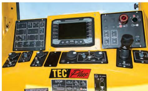
**SMARTTEC ELECTRONIC CONTROL SYSTEM.** SmartTEC performance software helps optimize productivity with real-time machine control prompts. Monitor and record functions encourage proactive machine maintenance and operator performance analysis. Available on all Vermeer TEC® Plus system-equipped machines.
