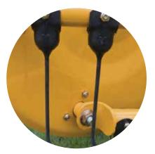
6 Six bar baskets on the R2300 (seven bar baskets on the R2800) mean maximized sweeping action, especially in high-volume conditions. Rubber-mounted tines can help reduce maintenance and service time.
