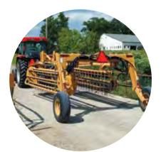
5 Transportation is fast and convenient. Hydraulic control from the cab allows operators to navigate narrow gate openings and country roads with transport widths of 8.4 ft (2.6 m) on the R2300 and 8.5 ft (2.6 m) on the R2800.
