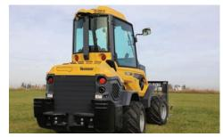
**COMPACT SIZE.** With narrow tires, the ATX960 is 52 in (132 cm) wide, while the wider tires make the machine 59 in (150 cm) wide. Both configurations allow the ATX960 to fit through many standard gates for backyard access. The overall length of the ATX960 is 126 in (320 cm).
