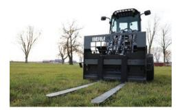
LIFT-CAPACITY-TO-WEIGHT RATIO. The ATX960 has a rated operating capacity of 3,285 lb (1,490 kg) with 970 lb (440 kg) back weights while having a standard weight of 4,720 lb (2,140 kg). This lift-capacity-to-weight ratio allows contractors to utilize a lighter machine while still being able to carry heavy materials on the jobsite.
