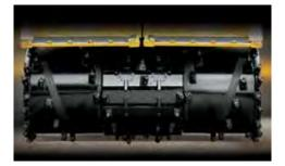
**CHAIN DRIVE TERRAIN LEVELER SEM** ATTACHMENT OPTION. The chain drive Terrain Leveler option gives you the capability to cut along a vertical high wall, with a maximum cutting depth of 27" (68.6 cm).
