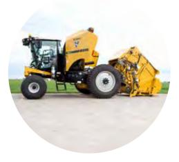
6 By automating parts of the baling process, the ZR5-1200 helps reduce the number of manual steps to make a bale to just one step. When you choose to bale in automatic mode, the ZR5-1200 control system, paired with a hydraulic drive system, can make realtime adjustments based on field and crop conditions and can even open and close the tailgate automatically.
