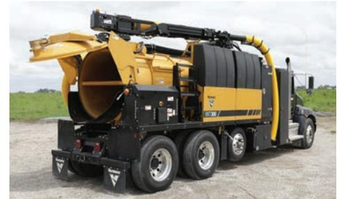
**CAM-OVER REAR DOOR.** The highly reliable cam-over design provides a 360-degree positive seal, with no additional clamping and no in-tank moving parts.
