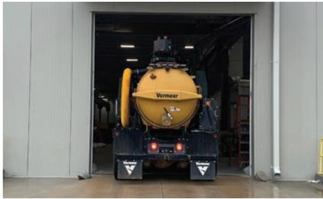
**LOW PROFILE.** Low overall height of 11.5 ft (3.51 m). Drive under a 12-ft (3.66-m) shop door or bridge with comfort. Plus, one of the lightest 8-yd<sup>3</sup> (6.1-m<sup>3</sup>) trucks in the industry to maximize payload.
