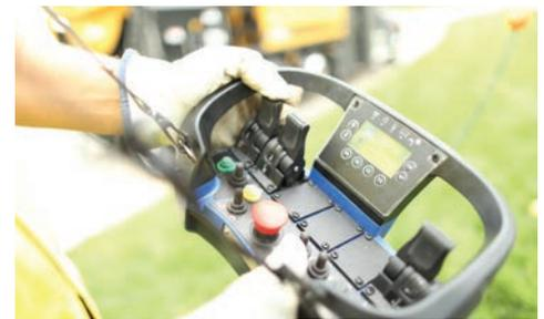
**INNOVATIVE CONTROL SYSTEM.** Choose from durable full-function belly-pack or handheld remote. Innovative control system allows for one-person operation.
