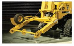
5,000 LB REEL CARRIER ATTACHMENT OPTION. On the tractor equipped with a plow, add a reel carrier attachment capable of carrying up to 5,000 lbs of product.
