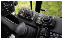
PRODUCTIVITY PACKAGE. Cut trenches confidently and efficiently with TrenchSense™ electronic control system, EcoldleTM engine control system, Productivity Zone, and Auto Plunge. Continuously cut with a sod knife designed to minimize buildup and keep you running.
