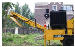
**FOLDING DISCHARGE CONVEYOR.** 7 ft (2.1 m) discharge height. Facilitates ease of transportation.
