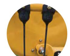
6 Six bar baskets on the R2300 (seven bar baskets on the R2800) mean maximized sweeping action, especially in high-volume conditions. Rubber-mounted tines can help reduce maintenance and service time.
