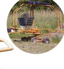
With a transport width of 6.6 ft (2 m), the RR140 has perimeter guarding on both sides, which folds directly up, and the 11 arms hook into storage locations on the tongue. This provides the ability to transport on narrow roads and through gate openings.
