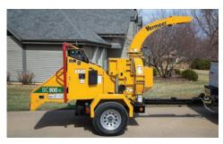
**EASE OF SERVICE.** This machine offers direct access to all parts of the chipper for routine maintenance without having to climb on or remove any shields. A dripless oil filter and five grease points are provided to reduce work effort and speed up service time.
