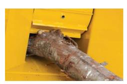
LARGE RECTANGULAR FEED OPENING. The large 9 in x 14 in (22.9 cm x 35.6 cm) feed opening helps boost productivity by reducing the need to trim heavily branched material before feeding it into the chipper.
