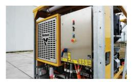
REMOTE LOCKOUT. The SA2500E can be activated and deactivated from a remote when connected to a Vermeer drill.
