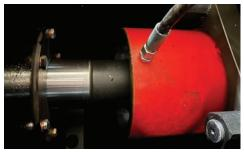
**SCALABLE.** Depending on the diameter of the liners, the SA2500E can deliver up to 3.100 L/min at 60 bar, covering a wide range of applications. The standard configuration comes with 7-in liners, delivering 2.400 L/min at 80 bar.
