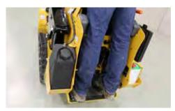
**ENJOY THE RIDE.** A dedicated spring-cushioned platform keeps the operator out of the mud. The integrated operator presence system suspends ground drive and powered boom/bucket motion when the operator steps off the platform.
