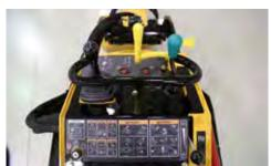
STEADY TURNS. A single, pilot-operated ground drive joystick offers a smooth range of motion without balancing engagement of two separate controls.
