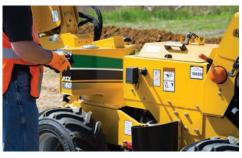
**REMOTE CONTROL.** When plowing or in transport mode, remote control operation offers flexibility in congested areas, providing the operator both fingertip control and smooth machine handling. The remote control functionality provides adjustability for the operator to maintain visibility to the work area and machine operation from a variety of viewpoints. When trenching, the operator controls utilize a tether that connects the machine and remote control.
