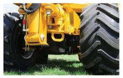
**TRACTION OPTIONS.** With a variety of different traction options, the PTX40 is well-suited to contractors' differing needs. The 23 in (58.4 cm) tire option is best for narrow, congested jobsites, the 26 in (66 cm) tire option provides better traction, and the dual tire option accommodates lower ground pressure requirements. Additionally, the PTX40 is available with tracks which are ideal for uneven terrain.
