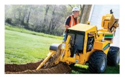
**COMPACT SIZE.** At minimum 40.2 in (102.1 cm) wide and only 55 in (139.7 cm) high, the PTX40 is small enough to navigate smaller jobsites where larger machines can't fit.
