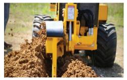
**MACHINE VERSATILITY.** Utilized for irrigation and utility installations, the versatile PTX40 is a plow/trencher with a dedicated plow depth of up to 24 in (61 cm), a trench depth of up to 42 in (106.7 cm) and a width of 4–6 in (10.2–15.2 cm). The optional bore attachment has a maximum torque of 494 ft-lb (670 Nm).
