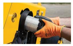
**SERVICEABILITY.** Access to required service points, as well as fuel, hydraulic oil, engine oil and air filters, does not require removal of any shielding, which can increase efficiency of machine service and simplify daily maintenance.
