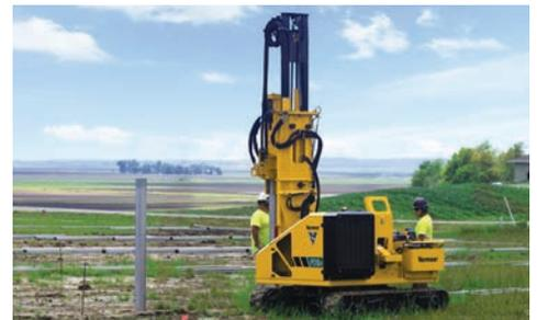
**KEEP IT LIGHT.** The PD5R weighs in at 10,300 lb (4672 kg), which allows for transporting up to two pile drivers on select trailers, and less potential damage to jobsites, all while helping increase efficiency of setup and teardown with a lightweight design.
