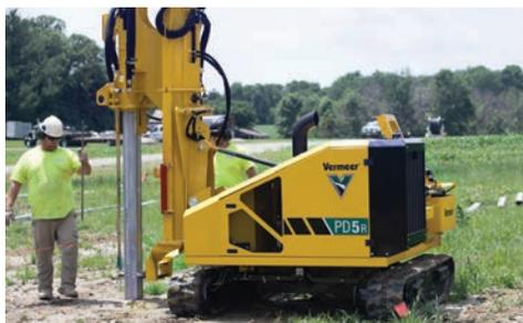
**COMPACT DESIGN.** A small machine with operating dimensions of 12.5' (3.8 m) wide, 19.6' (6 m) tall and a 15' (4.6 m) mast is ideal for jobsites with less space, or for multiple smaller jobs that require continual transportation of the machine. Quickly move around the jobsite and continue efficiency of installations, helping reduce time spent on setup, teardown and transportation.
