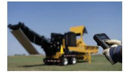
**COMPLETE CONTROL.** Optimize productivity and flexibility when operating the grinder with these two features: An industry-leading, full-function, wireless remote control lets you adjust machine settings from the cab as conditions change, including control of the infeed settings, engine droop, conveyor height and more. The 7-in (17.8-cm) onboard color touch screen display shows machine data and allows you to intuitively set up the machine for maximum efficiency.
