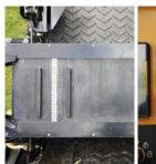
**CONTAMINATION DEFENSE.** Machine damage caused by metal contaminants entering the hammermill can be costly. The Vermeer Damage Defense system helps protect your machine by detecting certain metal contaminants, which reduces the likelihood of metal being processed by the hammermill. Combined with the cross-band magnet that minimzes metal from ground material, you can maximize the value of your end product.
