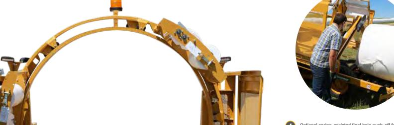
4 Optional spring-assisted final bale push-off feature smoothly ejects the last bale from the wrapper.
