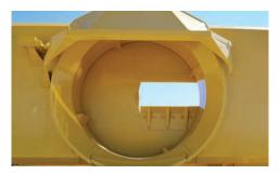
JOBSITE SAFETY. The thrown object restraint system (TORS) reduces the amount and distance of thrown material debris and has a smooth underside for optimal material flow.
