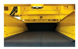
**HIGH PRODUCTION.** Smooth, 63-in (160-cm) belt enables high-volume product removal and is constructed of .5-in (1.3-cm) thick rubber to help resist tearing and puncturing.
