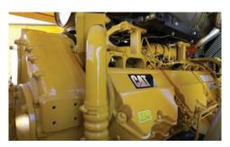
ENGINE POWER. A CAT C32 Tier 4 Stage V engine provides 1,125 hp (838 kW) of power to meet your jobsite demands.
