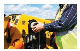
**SERVICEABILITY.** Access to hydraulic, engine oil and air filters does not require removal of any shielding, which makes machine service and preventive maintenance more efficient.
