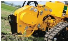
**MAXIMUM PRODUCTIVITY.** The dedicated plow has a maximum installation depth of 24 in (61 cm), while the optional trencher attachment has a maximum trenching depth of 42 in (106.7 cm) and width of 6 in (15.2 cm).
