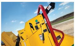
**EASILY LIFTS HEAVY MATERIAL.** An optional winch allows operators to move large logs effortlessly. The 150 ft (45.7 m) winch line can handle logs up to 2000 lb (907.2 kg) and can be used to lift the log onto the feed table.
