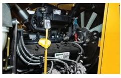
**ELECTRONIC FUEL INJECTION ENGINE.** With improved fuel economy, the 135 horsepower (101 kW) Power Solutions International (PSI) engine allows for more efficient working conditions and boosts engine response under load.
