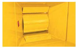
**DUAL HORIZONTAL OFFSET FEED ROLLERS.** Improve performance by aggressively grabbing and feeding material to the drum. The offset helps the upper feed roller climb over big logs or material with lots of branches and forks.
