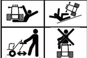
**WARNING:** Runover/Rollover can crush.
