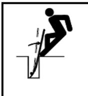
**WARNING:** Serious injury or death is possible if struck by guide tool. Never use hands, feet, shovel, rake, or other tools to manually assist the boring attachment.
