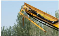
FOLDING DISCHARGE CONVEYOR. 7 ft (2.1 m) discharge height. Facilitates ease of transportation.
