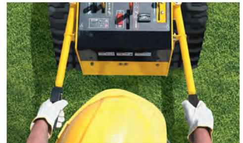
**VZ STEERING.** Instead of additional levers and steerable wheels, the operator can turn the machine using only the handlebars. These bars also provide additional leverage when operating in difficult terrain.
