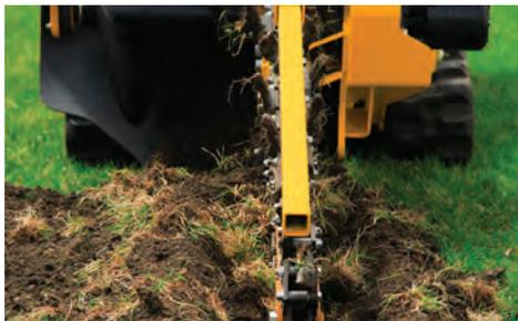
**OUTBOARD BEARING SUPPORT:** This feature provides protection for the headshaft when trenching in difficult conditions, helping to lower the overall cost of operation.
