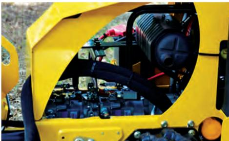
**OPERATORS, START YOUR ENGINE.** The 25 hp (19 kW) Kohler electronic fuel-injected (EFI) gasoline engine offers improved fuel economy reducing greenhouse gas by an average of 25 percent — as compared to conventional carbureted engines. And, best of all, makes choke cables obsolete. Simply put, it's time to start your trencher like you would your car.
