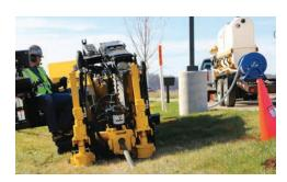
NEED FOR SPEED. With a carriage speed of 206 ft/min (62.8 m/min) and a rotational speed of 219 rpm, the D23x30 S3 helps contractors install more linear feet per day, maximizing jobsite productivity and efficiency.
