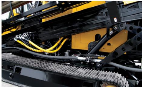
**INCREASE YOUR RANGE.** Unique four-bar linkage rack and additional pads allow operators to set up entry angles of 11° – 24° — increasing range attainable with tracks fully on ground.
