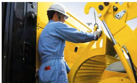
**SIZING FLEXIBILITY.** The top-loading design provides easy access to change screens, and a variety of screen sizes are available to meet your needs.
