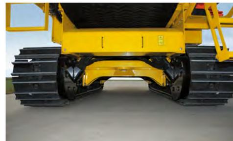
**MOBILITY.** The track-driven grinder offers onsite mobility with a remote control. The HG4000Tx is designed with 16" (40.6 cm) of ground clearance, enhancing the unit's ability to traverse difficult terrain.
