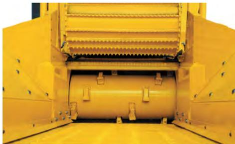
**OPTIMAL CUTTING PERFORMANCE.** The hardfaced duplex drum offers proven cutting performance, and reversible hammers and tips nearly double the wear life of single-sided designs and simplify daily maintenance. The optional chip drum produces a consistently chipped end product, rather than traditional shredded material, for uses such as biofuel.
