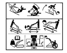
**WARNING:** Traveling on slopes or with load elevated may result in tip over. Serious crushing injury or death can result.
