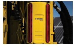
**MAINTAIN ACCURACY.** The PD5 has an optional laser receiver and an optional compatible third-party GPS system that can provide visual input to the operator, which can help improve productivity and alignment of the machine to the specified pile location.
