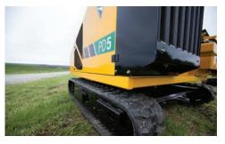
**MOVE ALONG.** With a forward ground drive speed of 2.4 mph (3.9 km/h), the PD5 moves quickly around the jobsite with less time wasted traveling and more time installing piles - keeping your installation efficiently moving forward.
