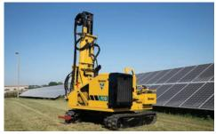
**KEEP IT LIGHT.** The PD5 weighs in at 10,380 lb (4,708 kg), which allows for transporting up to two pile drivers on select trailers, and less potential damage to jobsites, all while helping increase efficiency of setup and teardown with a lightweight design.
