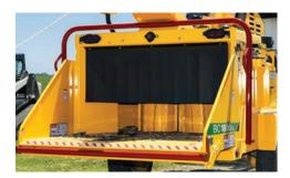
**OPERATOR SAFETY.** Mounted over the feed table, the four-position upper feed control bar enables the operator to stop the feed rollers and select forward or reverse. The patented bottom feed stop bar is strategically located to make it possible for an operator's leg to strike the bar and shut off the feed mechanism either intentionally or automatically in an emergency situation.
