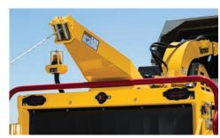
**EASILY LIFT HEAVY MATERIAL.** An optional winch allows operators to move large logs effortlessly. The 150 ft (45.7 m) winch line has 2000 lb (907.2 kg) pulling force and can automatically lift the log onto the feed table. With the chain choker detached it is also more easily attached to log than hook-on cable designs.
