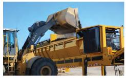
**CONVENIENT LOADING.** Large, low-feed hoppers are easier to load without the need for loading ramps.
