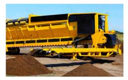
**RADIAL STACKING CONVEYOR.** Simple stacking conveyor with 180° arc increases the amount of material being stacked on the ground. Adjustable stacking height aids with dust control and helps avoid material being blown away.
