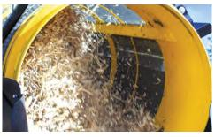
**HIGH PRODUCTION.** The tensioned screens around the drum add rigidity, allowing use of smaller-gauge wire — which helps increase production capacity and enable processing of wetter material.
