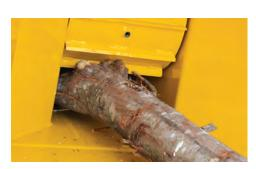
LARGE RECTANGULAR FEED OPENING. The large 9" x 14" (22.9 cm x 35.6 cm) feed opening helps boost productivity by reducing the need to trim heavily branched material before feeding it into the chipper.
