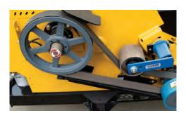
**CENTRIFUGAL CLUTCH.** The centrifugal clutch engagement prevents belt slip when engaging the clutch which means fewer maintenance costs.
