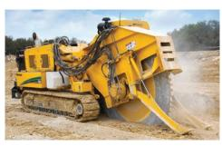
**HYDROSTATIC ROCKWHEEL ATTACHMENT.** Powered by a hydrostatic motor, the optional rockwheel attachment has the ability to cut a trench up to 4' (1.2 m) in depth and 10" (25.4 cm) in width.
