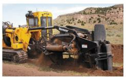
**OPTIONAL BUCKET WHEEL ATTACHMENT.** Designed for the installation of small-diameter cross country pipelines in soft digging conditions, the attachment has the ability to cut 22", 24" or 28" (55.9 cm, 61 cm or 71.1 cm) wide trenches.
