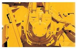
**ROTARY POWER TRENCHER DRIVE MOTOR.** A rotary power trencher drive motor and splined headshaft produce a lower speed and higher torque, which provide superior ground penetration and low chain wear for better production results.
