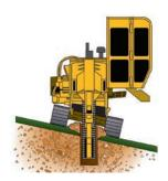
**OPTIONAL AUTO TILT TRACK.** An oscillating track frame allows the track to follow the ground's contour, providing a vertical trench on slopes up to 10.5 degrees.
