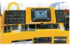
**SMARTTEC ELECTRONIC CONTROL SYSTEM.** SmartTEC performance software helps optimize productivity with real-time machine control prompts. Monitor and record functions encourage proactive machine maintenance and operator performance analysis. Available on all Vermeer TEC<sup>®</sup> Plus-equipped machines.
