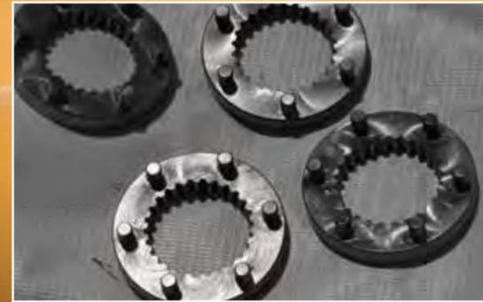
The Quick-Change shear ring is a small ring with pins that sits within the disc hub. Pins shear when the disc encounters a potentially damaging obstacle to help protect the internal gears and drive spline, while the hub retains the disc. Operators replace the ring rather than the hub, reducing potential contamination to the cutter bar.
