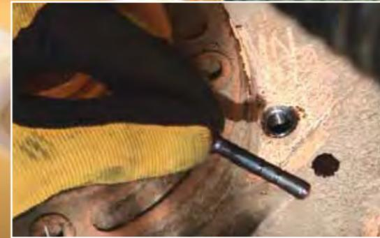
The Q3 cutter bar has a quick-check system with a built-in dipstick to check oil levels of the individual cutter units.
