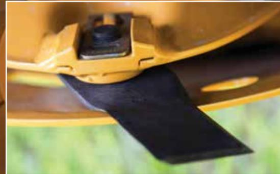
The Quick-Clip system allows operators to quickly replace or reverse blades. Slide out the clip, reload the new blade, tap it in place with the provided tool and get back to mowing.
