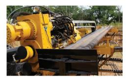
ROD LOADER. A single row, sliding arm rod loader allows for the staging of five rods at one time, increasing boring efficiency by minimizing rod loading time.
