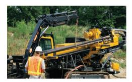
KNUCKLEBOOM CRANE. The optional knuckleboom crane mounted on either side of the base anchor maneuvers heavy tooling, reducing the need for support equipment.
