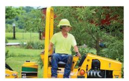
JOBSITE VISIBILITY. The operator's station is located at the center of the service plow directly above the machine's articulation point, which provides excellent visibility of the entire work area.
