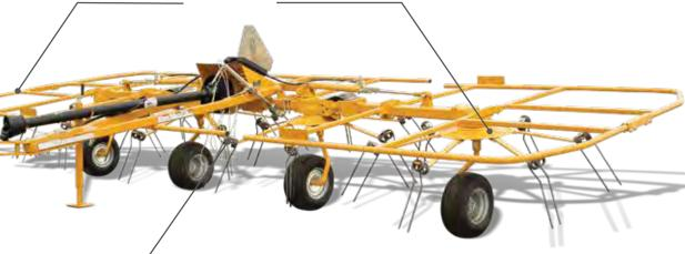
3 The transport lock on the TD190 can be released from the tractor seat, and the outside rotors can hydraulically fold to a 10.9-ft (3.3-m) transport width, making it convenient to quickly move from field to field.
