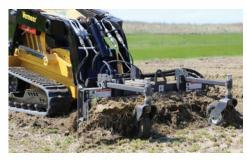
**DUAL HYDRAULIC SYSTEM.** The CTX160 dual hydraulic system is capable of providing 16.7 gpm (63.2 L/min) of hydraulic flow, powering demanding attachments. Low flow offers 9.4 gpm (35.6 L/min) to give maximum control.
