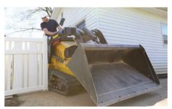
**COMPACT FOOTPRINT.** This unit is designed to get through standard residential gates and into tight access areas. With 9-in (22.9 cm) tracks, the CTX160 is 42 in (106.7 cm) in total width. Offering maximized traction and low ground pressure.
