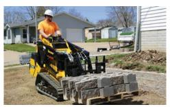
HIGH-CAPACITY LIFTING. The vertical lift capability on the CTX160 boasts a rated (SAE) operating capacity of 1,600 lb (725.7 kg) and a hinge pin height of 88.75 in (225.4 cm).
