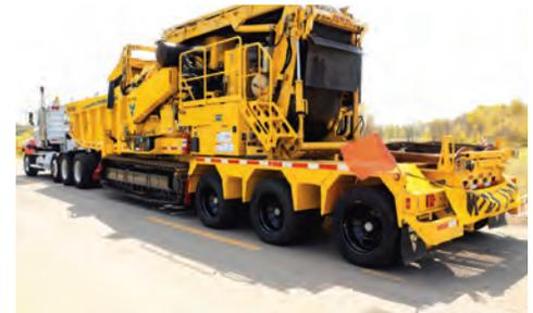
**MOBILITY.** The track-driven grinder offers onsite mobility, with a remote control for easy maneuverability. The DT6 optional integrated dolly transport system eliminates the need for a dedicated trailer to move between sites.
