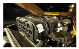
POWER FOR THE JOB. Take on difficult ground conditions with the efficient power of a 127-hp (95- kW) Deutz TCD3.6L diesel engine.
