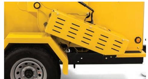
**LARGE FEED OPENING.** The BC1000XL features a 12" (30.5 cm) tall and 17" (43.2 cm) wide infeed opening. This design can help boost productivity by decreasing the amount of trim cuts needed prior to processing.
