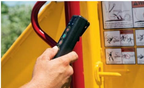
**TAKE CONTROL.** With the standard Tree Commander™ remote control, jobsite productivity is improved by allowing the operator to control brush chipper functions remotely. The remote can be attached to the operator's belt or held in an optional bracket mounted directly to the operator's station of a Vermeer mini skid steer.
