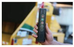
CONTROLLED JOBSITE. The Tree Commander™ remote comes standard with the BC1800xL gas to help with productivity on the jobsite and let the operator control the brush chipper functions remotely. The remote can be attached to the operator's belt or held in an optional bracket mounted directly to the operator's station on a Vermeer mini skid steer.
