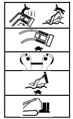
**WARNING:** Abrupt movement and uneven terrain can throw operator off machine.
